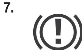
Brake System Warning
